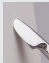
The winged elevator tip is placed flat against the sharpening stone
