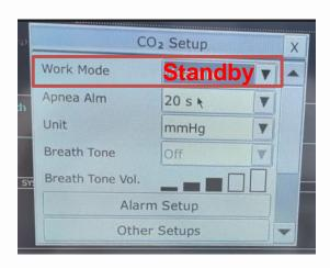
In standby mode, the EtCO2 module stops working. The pump rests and it stops sampling.
