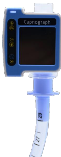
Figure 8. Capnograph connected to an endotracheal tube
